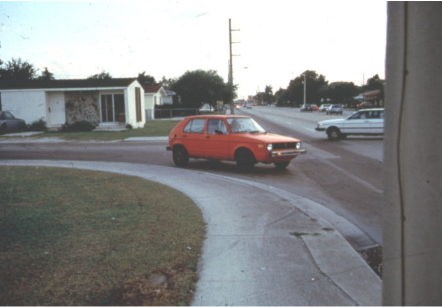
HAZARDOUS FOR PEDESTRIANS: CONVENTIONAL CURB RADIUS REQUIREMENTS ALLOW CARS TO SPEED AROUND CORNERS WITHOUT SLOWING DOWN.
