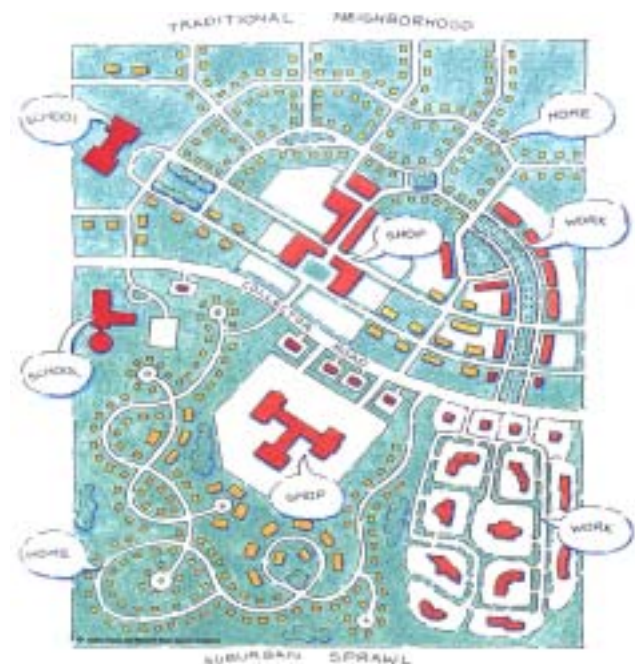
SPRAWL (BELOW) VS. THE TRADITIONAL NEIGHBORHOOD (ABOVE): IN CONTRAST TO THE TRADITIONAL NETWORK, THE SPRAWL MODEL'S CUL-DE-SAC ORGANIZATION FOCUSES ALL TRAFFIC ONTO A SINGLE ROAD.
