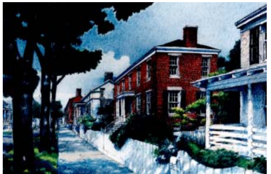
NIAGARA-ON-THE-LAKE, ONTARIO: A RANGE OF SHORT SETBACKS (15', 10', 5', AND 0' ) PROVIDE VARIETY WHILE DEFINING THE STREET EDGE.
