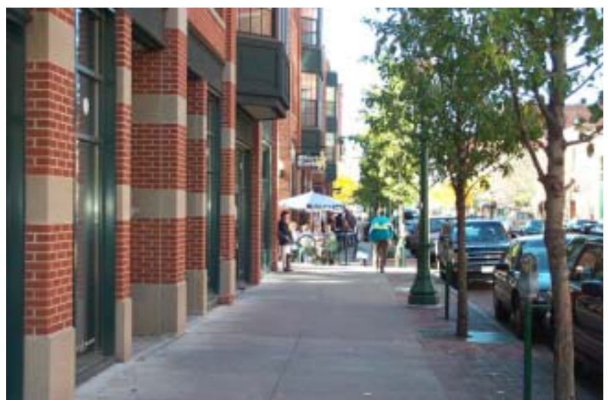
ARMORY SQUARE: STREETLIGHTS, SIGNPOSTS, FIRE HYDRANTS, AND TREES ARE ALL LOCATED TOWARD THE OUTER EDGE OF THE SIDEWALK.
