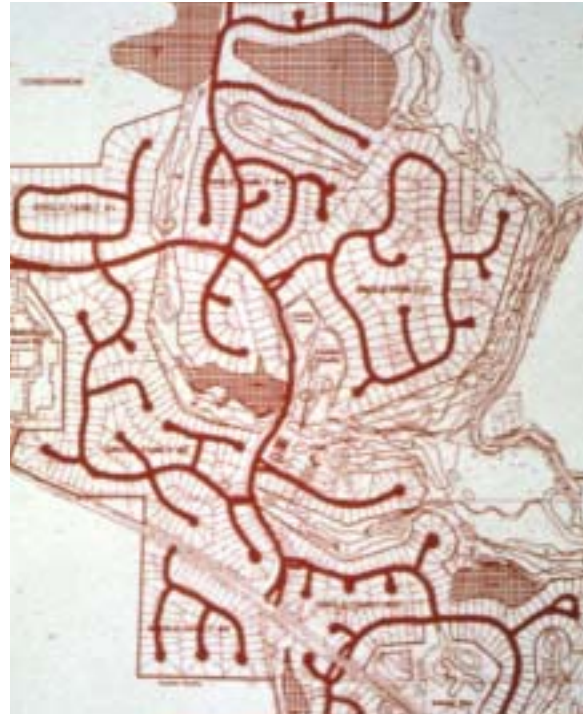
CONFUSING BY DESIGN: CONVENTIONAL SUBDIVISION PLANS DISORIENT VISITORS WITH OVERLY CURVY STREETS.
