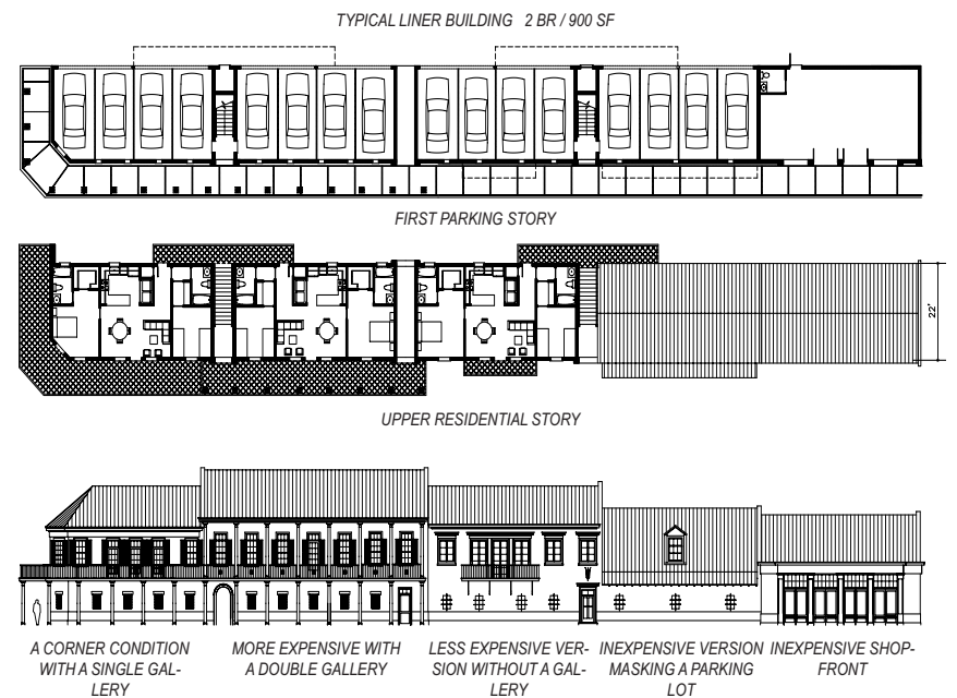
THE LOT-LINER: TO HIDE PARKING LOTS IN BATON ROUGE, A NEW BUILDING TYPE WAS INTRODUCED THAT PLACES AFFORDABLE APARTMENTS ABOVE PARKING SPACES.
