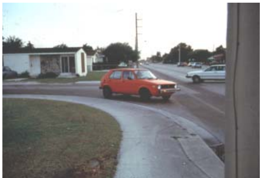
HAZARDOUS FOR PEDESTRIANS: CONVENTIONAL CURB RADIUS REQUIREMENTS ALLOW CARS TO SPEED AROUND CORNERS WITHOUT SLOWING DOWN.
