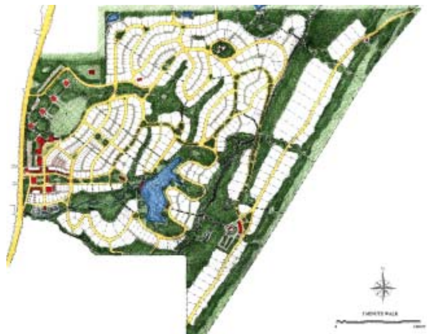
MOUNT LAUREL, ALABAMA: THE WINDING ROADS, QUIRKY INTERSECTIONS, AND VARIED DENSITY ALL AROSE FROM THE GOAL OF PRESERVING THE EXISTING TOPOGRAPHY.
