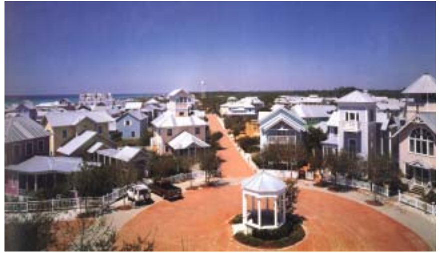
TRAFFIC-CALMED: AT SEASIDE, A ROUNDABOUT, SHARP CORNERS, AND 16'-WIDE STREETS KEEP CAR SPEEDS DOWN.
