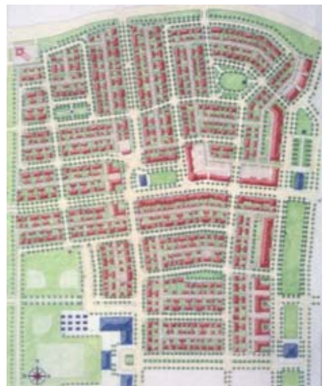
THE STREET NETWORK IN A CORNELL NEIGHBORHOOD: A RICH HIERARCHY THAT EMPHASIZES THE CENTER AND EDGES.
