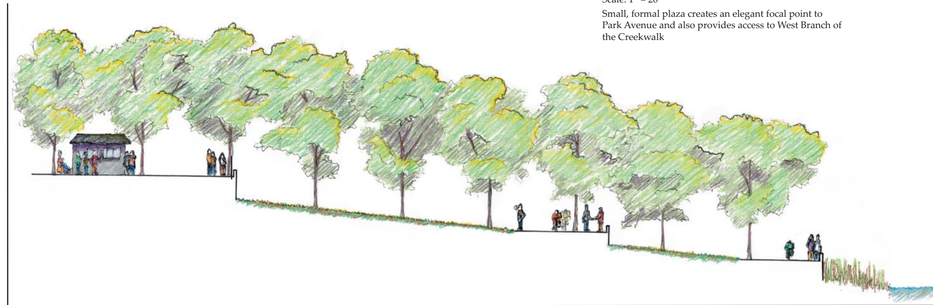
Section C: Tracy Street Extension Scale: 1" = 20' Series of platforms refer to historic alignment of Tracy Street while creating gathering and viewing areas.
