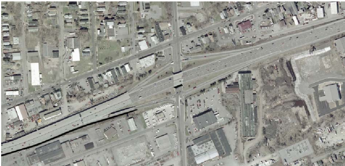
Figure 5.3: Typical Diamond Style Interchange. Route 690 and Teal Avenue Intersection. Source: New York State Geographic Information Systems, 2003.
